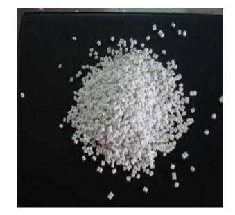
Filler master batch is a Calcium carbonate based polymer additive used in Film, raffia bags and molded products. When added to the formulation, reduces the production cost whilst retaining the required properties of the product. Different grades of filler additives are on offer for Opaque/color Film, transparent matt film, glossy film, lamination, molded products and raffia bags.
