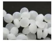
Antiblock masterbatches counter acts the tendency of extruded films in sticking together and helps in improving the opening characteristics of films/bags. Its applications include mono / multilayer blown film for flexible packaging.
