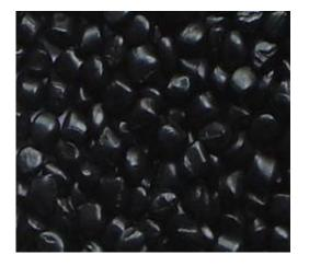
The performance of black masterbatches primarily depends on the dispersion of carbon black in the carrier
