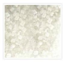
Slip masterbatches prevent blocking of adjacent Polyolefin film surfaces to each other when brought into contact together during manufacturing such as blown film production. It reduces the co-efficient of friction of the polyolefin film surface very smoothly, ensuring superior handling properties and doesn't affect the sealing and printing properties. Primary application of Slip masterbatches is in mono / multilayer films etc.
