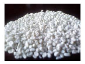
Antistatic Masterbatch is used to reduce the electrical resistance on the surface of films and molded products. It also gives uniform cell size distribution in expanded polyethylene (EPE) foams. It offers electrical properties spanning the surface resistivity spectrum from 1010 to 1013 ohm/sq and sustains for a long period. Its applications include packing in medicine, electronics. It can also be used in extrusion process to avoid static charge.
